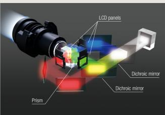
All three colors are simultaneously projected onto the screen, delivering brighter, more vibrant images.
